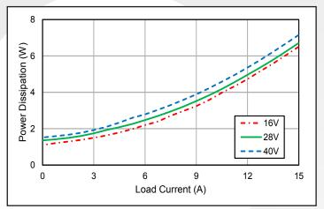
*Figure 3:* Power dissipation at nominal output voltage vs. load current for minimum, nominal, and maximum input voltage at  $T_{css}=25^{\circ}C$ .
