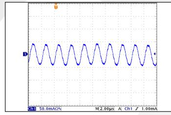
**Figure 9:** Input terminal current ripple, i<sub>c</sub>, at full rated output current and nominal input voltage with SynQor MCOTS filter module (50 mA/div). Bandwidth: 20 MHz. Timescale: 2.00µs/div. See Figure 17.
