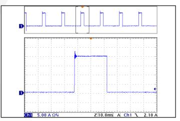
**Figure 18:** Load current (5A/div) as a function of time (10ms/div and 100ms/div) when the converter attempts to turn on into a 1 m $\Omega$  short circuit.
