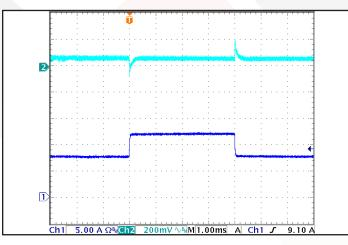
**Figure 11:** Output voltage response to step-change in load current (50-75-50% of Iout(max); dI/dt = 0.1 A/ $\mu$ s). Load cap: 1  $\mu$ F ceramic and 100  $\mu$ F electrolytic capacitors. Ch 1: Iout (5A/div), Ch 2: Vout (200mV/div). Timescale: 1.00ms/div.
