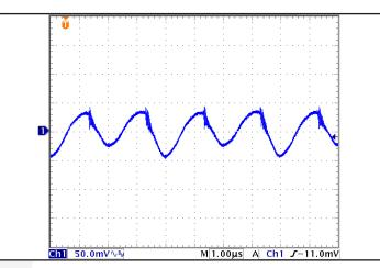
**Figure 10:** Output voltage ripple, Vout, at nominal input voltage and rated load current (50 mV/div). Load capacitance:  $1\mu$ F ceramic capacitor and  $15\mu$ F tantalum capacitor. Bandwidth: 20 MHz. Timescale: 1.00 $\mu$ sec/div. See Figure 17.
