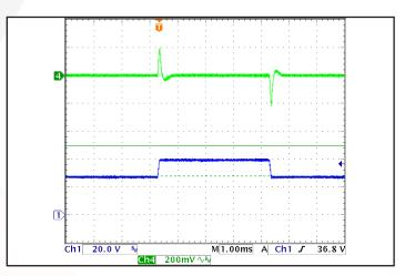
*Figure 12:* Output voltage response to step-change in input voltage (250V/ms). Load cap: 1uF ceramic and 15uF tantalum capacitance. Ch 1: Vin (20V/div), Ch 4: Vout (200mV/div). Timescale: 1.00ms/div.
