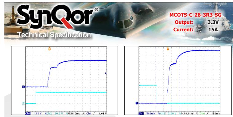
Figure 7: Turn-on transient at full load initiated by Nominal Vin. ON/OFF Pin previously low. Ch 1: Vout (1V/div). Ch 2: Vin (20V/div). Timebase: 10.0ms/div.
